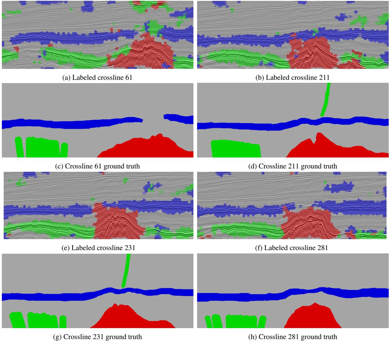
**Fig. 3:** Results of the proposed method on four different seismic sections in the Netherlands North Sea F3 block database [14]. The Chaotic class in blue, Faults is green, Salt dome is red, and Other is grey
