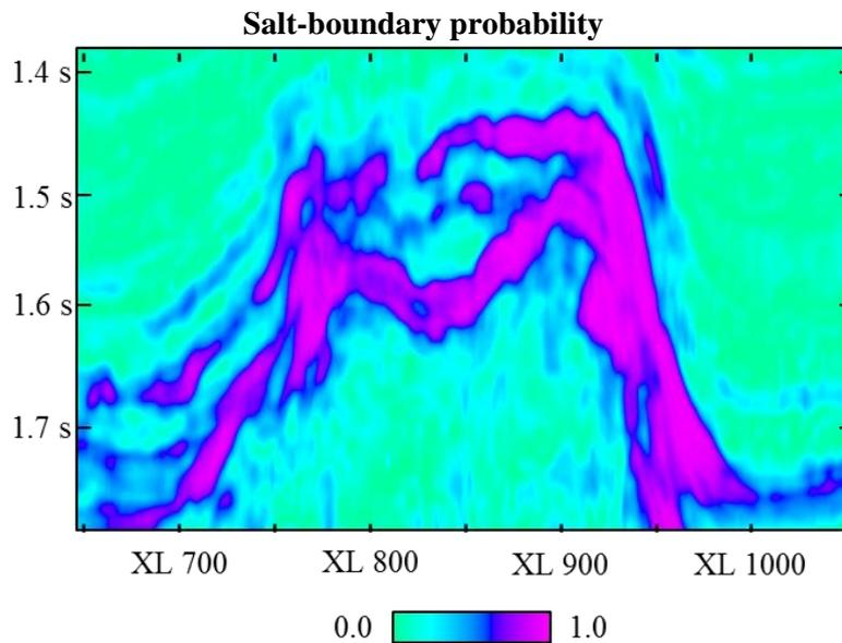
**Figure 3** The probability map of the salt boundaries generated by the proposed multi-attribute *k*-means cluster analysis for salt boundary detection.
