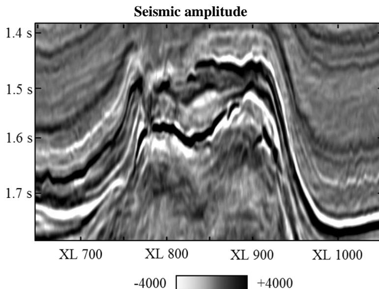
**Figure 2** The amplitude of the vertical section of inline 415 from the F3 block used for illustrating the proposed salt-boundary delineation method based on multi-attribute k-means cluster analysis.
