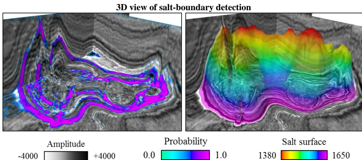
**Figure 4** 3D view of the detected salt boundaries (left) and the extracted salt surface (right) from the probability volume by the proposed multi-trace *k*-means cluster analysis.
