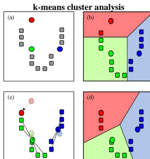
**Figure 1** The cartoon illustration of the k-means clustering of twelve observations into three clusters
