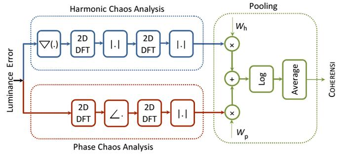
Fig. 1. Block diagram of the proposed similarity index, COHERENSI. Thick lines represent array signals, while thin lines represent scalar signals.
