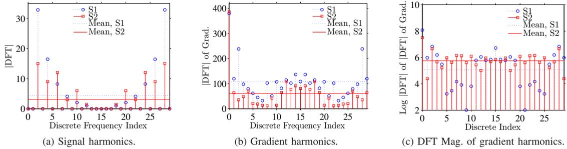
Fig. 2. Illustration of the ability of the proposed transform to differentiate between two signals with different harmonic behaviors.
