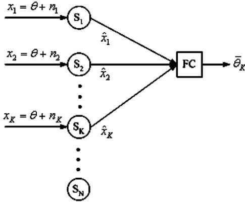
Fig. 1. Distributed estimation system under the total bit rate constraint.
