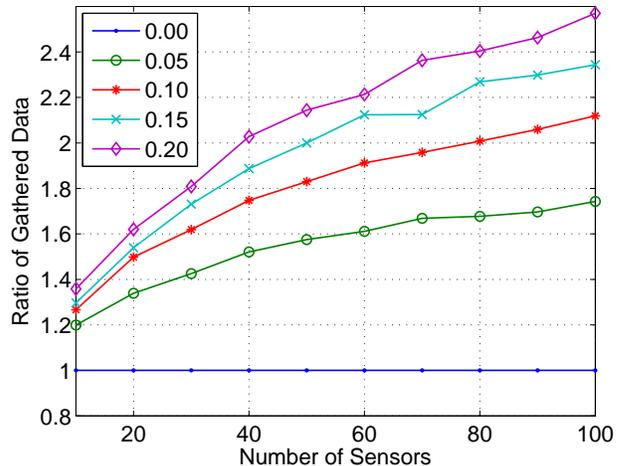
Fig. 2. Ratio of data volume gathered by the proposed algorithm to the heuristic method under different total number of sensors and different sensor noise variation parameters ( $\gamma = 0.00, 0.05, 0.10, 0.15, 0.20$ ).
