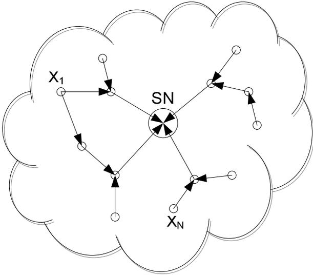
Fig. 1. An example of a wireless sensor network with  $N$  distributed sensor nodes. Each sensor makes observations on the sensor field and sends its sensed data to the sink node (SN) for further processing. In directed solid lines, a chosen multi-hop routing path is shown, where the data from a sensor can be relayed by multiple sensors, meanwhile a sensor can relay data for multiple sensors.
