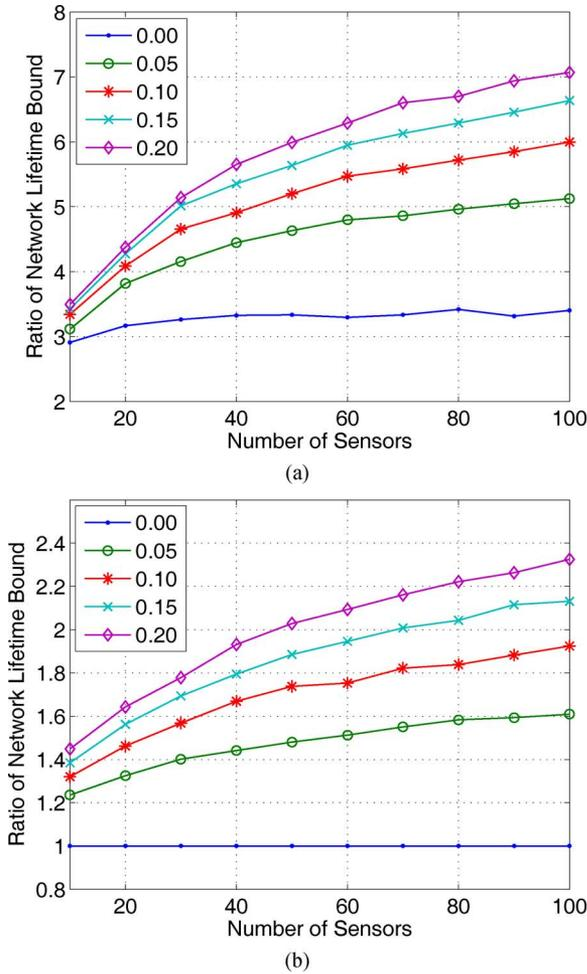
Fig. 4. Ratio of network lifetime bound by the proposed algorithm to that by two heuristic methods under different total number of sensors and different sensor noise variation parameters ( $\gamma = 0.00, 0.05, 0.10, 0.15, 0.20$ ): (a) compared with *Heuristic-I*, (b) compared with *Heuristic-II*.
