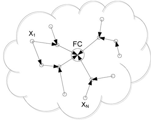
Fig. 1. An example of a wireless sensor network with  $N$  distributed sensor nodes. Each sensor can observe the phenomenon, quantize and transmit its observation to the fusion center (FC) via multihop wireless channel, and the fusion center makes the final estimation based on all the received messages. In directed solid lines, a chosen multihop routing path is shown, where the data from a sensor can be relayed by multiple sensors, meanwhile a sensor can relay data for multiple sensors.
