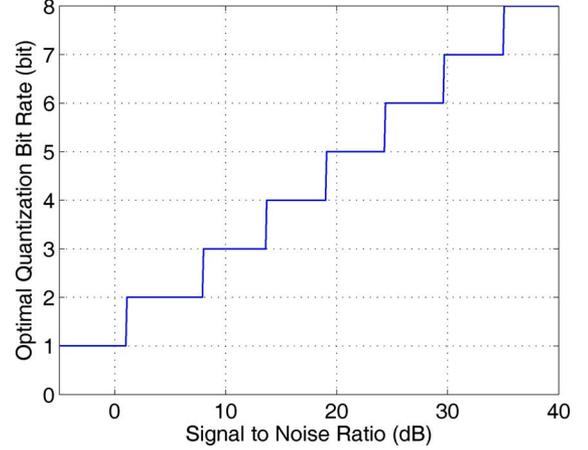
Fig. 2. Optimal quantization bit rate versus SNR.
