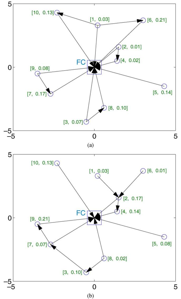
Fig. 5. The optimal multihop routing path for two example heterogeneous sensor networks with same sensor locations but different observation noise variances.
