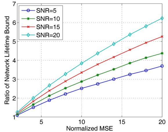
Fig. 3. Ratio of network lifetime bound for homogeneous sensor networks under different SNRs and normalized estimation MSE requirements.
