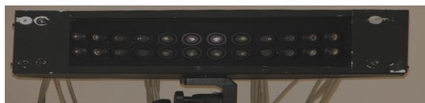
**Fig. 1.** The HP FanCamera is a 24-imager array mosaicking camera.
