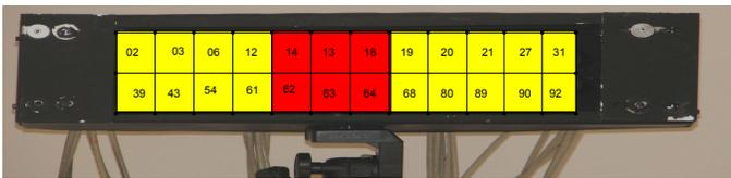
Fig. 5. The bit rate allocation in the uneven distribution coding experiments. The six middle cameras (in red) are considered the center of focus are allocated 80% of the bandwidth and 20% for the other cameras (in yellow).
