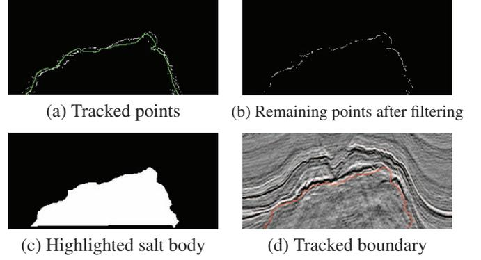
**Fig. 5:** The post-processing steps to synthesize the tracked boundary
