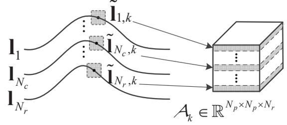
**Fig. 2:** The texture tensor built from the boundaries of reference sections
