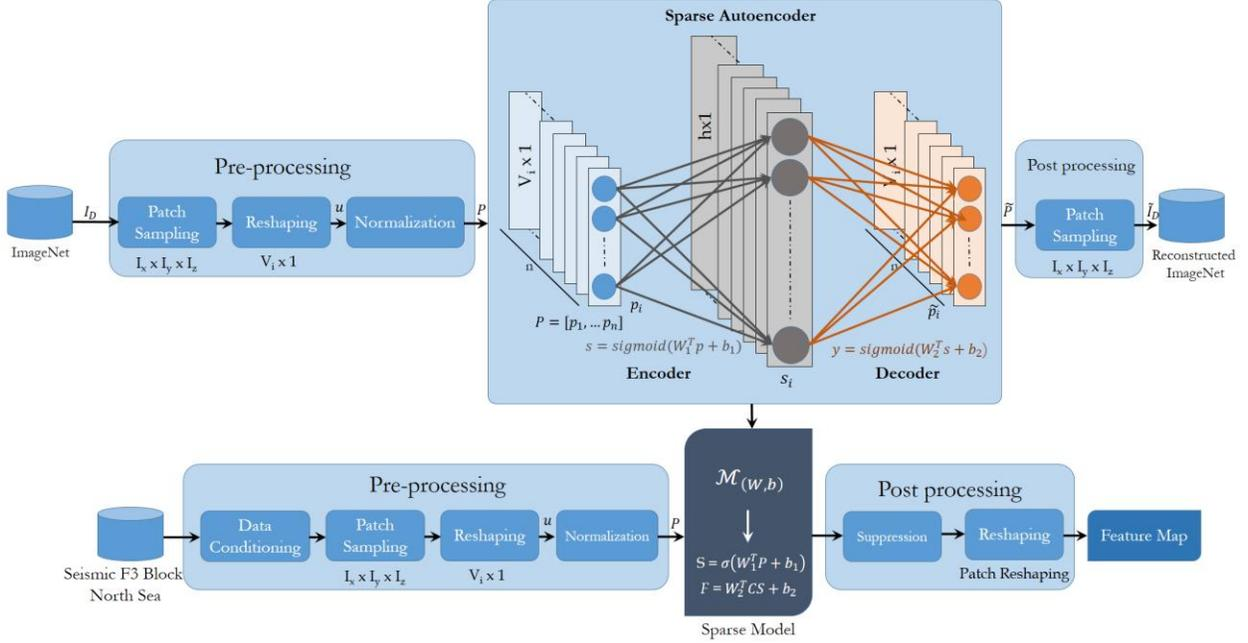
Figure 1: The block diagram of the unsupervised learning framework for seismic data analysis.
